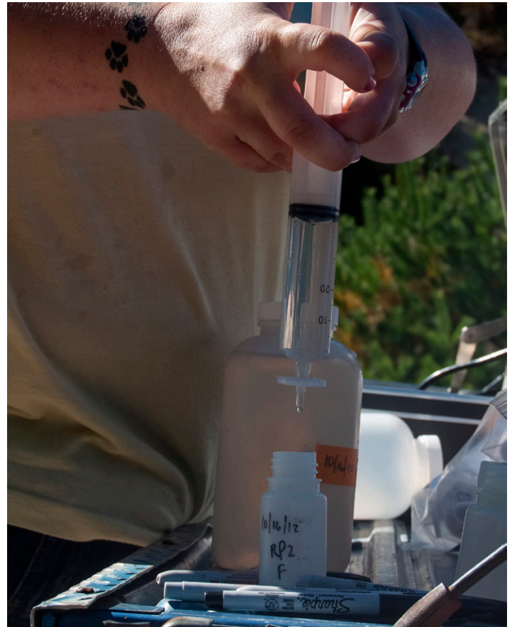
above Water samples collected from a bog are filtered prior to laboratory analysis for nitrogen and phosphorus.
